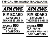
While lumber has been the traditional product used for Rim Boards, it is generally not compatible with the depth of the new generation of wood I-joists used in floor construction. With the increasing use of wood I-joists, a demand for compatible engineered wood Rim Boards has resulted.
