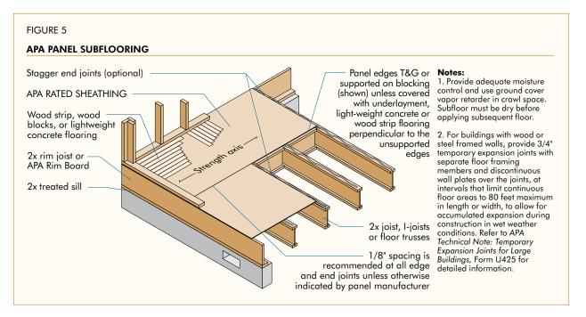
APA RATED SHEATHING Exposure 1 may be used where temporary exposure to moisture or weather is expected during construction. However, only Exterior panels should be used where long-term exposure to moisture or weather will be required. See "Plywood for Outdoor Decks" on page 89 for additional information on permanently exposed panels.
