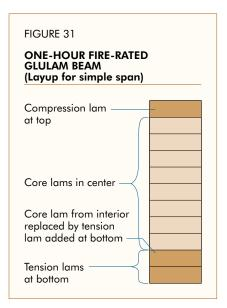
least one hour during standard ASTM E119 fire test conditions which simulate an actual fire.
