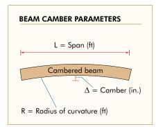
Camber for glulam beams is specified as either "inches of camber" or as a radius of curvature that is to be used in the manufacturing process. Commonly used curvature radii for commercial applications are 1,600 and 2,000 feet, although any camber may be specified.
