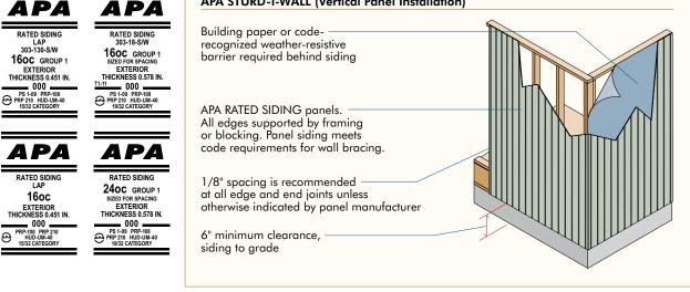
APA RATED LAP SIDING APPLIED DIRECT-TO-STUDS OR OVER NONSTRUCTURAL SHEATHING<sup>a,b,c,d,e</sup>
