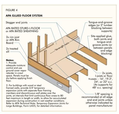
using ordinary construction materials and techniques. And like many other panel assemblies that provide excellent sound control, the APA Glued Floor System is ideal for multifamily construction. The large panels with glued tongue-and-groove joints reduce the number of cracks that can "leak" airborne noise.
