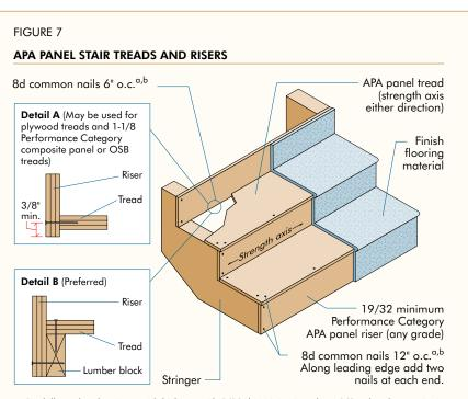
a. Predrill tread end grain at mid-thickness with 3/32" bit. Maintain at least 3/8" edge distance in riser. b. See Table 6, page 14, for nail dimensions.
