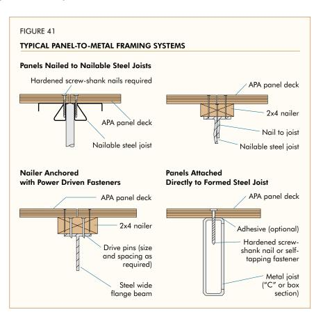
Typical panel-to-metal framing systems are illustrated in Figure 41. Load-span recommendations are the same as for wood-frame systems. For more information, refer to *APA Design/Construction Guide: Wood Structural Panels Over Metal Framing*, Form T625.
