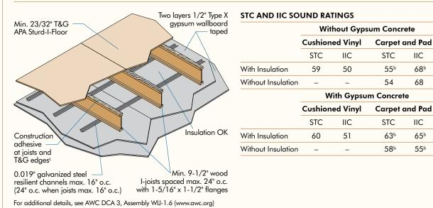
For other plywood floor-ceiling assemblies, see U.L. Design Nos. L506 (3/4 hr), L509 (1/2 hr), L520 (3/4 hr).
