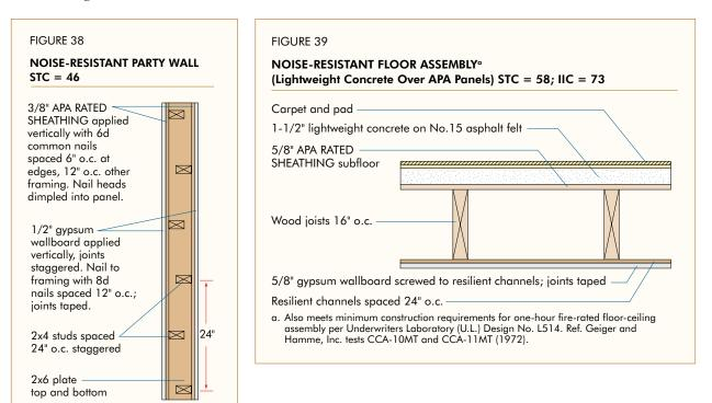
The IIC ratings define the capacity to control impact noise. In most cases, required IIC rating values are about the same as for STC.
